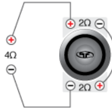
(1) 2 Ohm DVC Speaker = 4 Ohm Load
