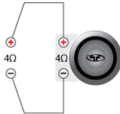
(1) 4 Ohm SVC Speaker = 4 Ohm Load
